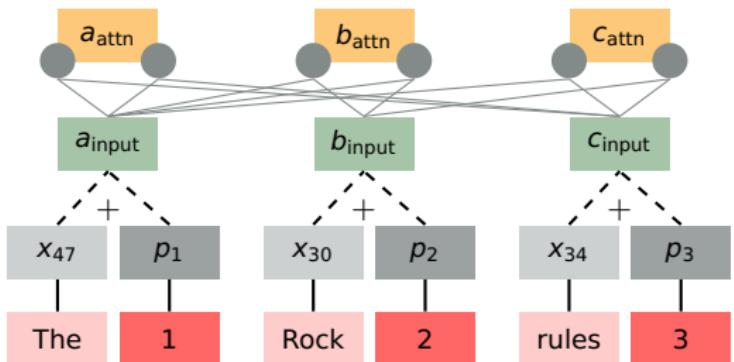
$$c_{\text{attn}} = \mathbf{sum}([\alpha_1 a_{\text{input}}, \alpha_2 b_{\text{input}}])$$
